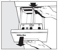
Pull out the detergent drawer until it stops. Press down on the red release lever and pull the drawer out of the machine.
